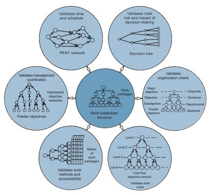
**FIGURE 11–3.** Work breakdown structure for objective control and evaluation. *Source:* Paul Mali, *Managing by Objectives* (New York: Wiley, 1972), p. 163. Copyright © 1972 by John Wiley & Sons. Reprinted by permission of the publisher.
