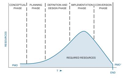
FIGURE 2–22. Definition of a project life cycle.
