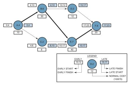
FIGURE 12–20. CPM network with slack.
