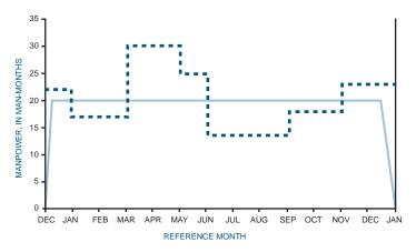
FIGURE 14–8. Typical manpower loading.
