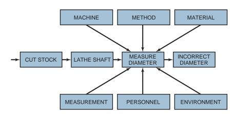
FIGURE 20–13. Process analysis method.
