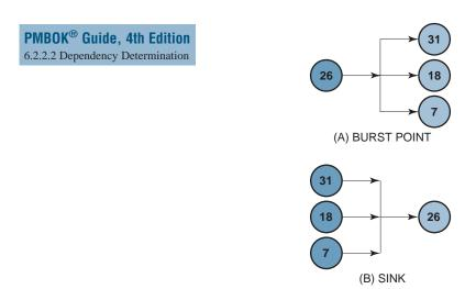
FIGURE 12–2. PERT sources (burst points) and sinks.
