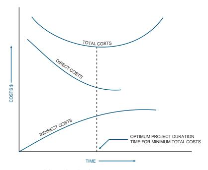
FIGURE 12–19. Determining project duration.
