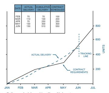
**FIGURE 13–14.** Delivery schedule tracking (line of balance).
