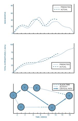
FIGURE 12-7. Comparison models for a time-phase PERT chart.
