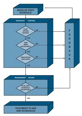
FIGURE 12–11. Iteration process for PERT schedule development.
