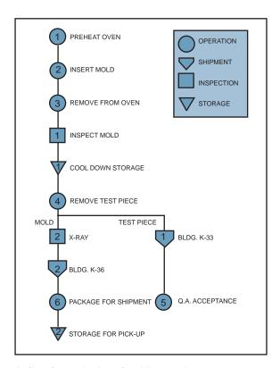
**FIGURE 13–15.** Logic flow for production of molding VZ-3.
