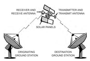
**FIGURE 25–1.** Typical satellite communication architecture.
