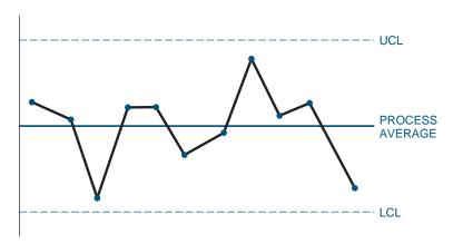
FIGURE 20-30. Process in control.
