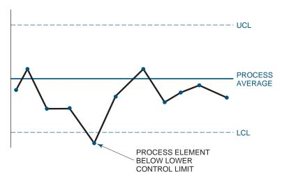
FIGURE 20-29. Control chart out of control.
