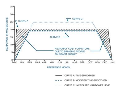
FIGURE 14-9. Linearly increased manpower loading.
