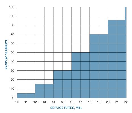
FIGURE 17–9. Step-function chart for random number service rates.
