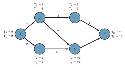
FIGURE 12-6. Network with slack time.
