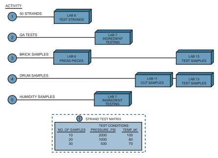
FIGURE 13-16. Propellant samples testing matrix.
